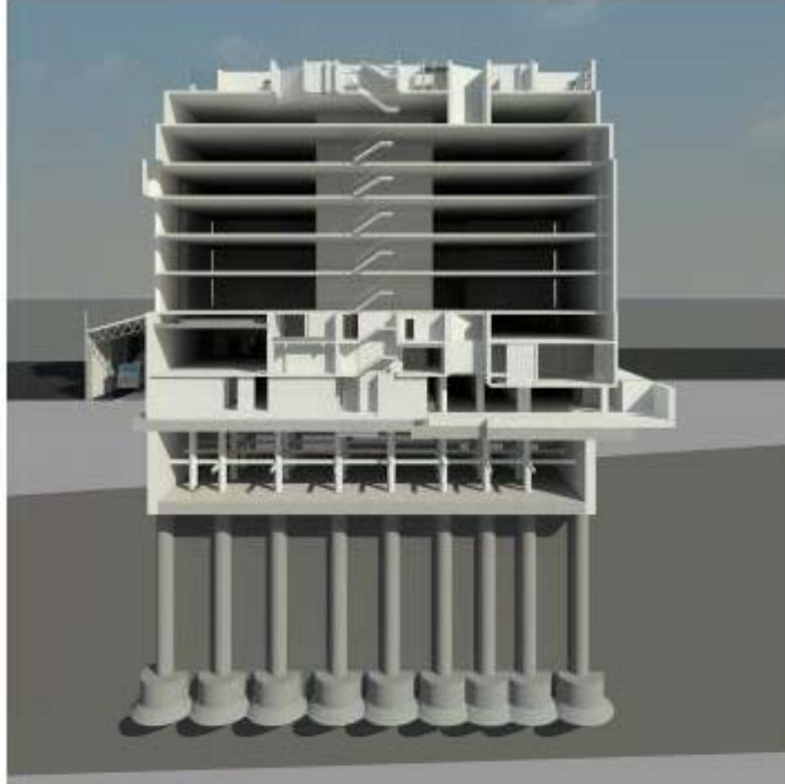
Current Consented Substructure
